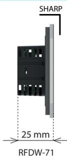
The glass design controller with two output relays is used to control appliances and lights.
